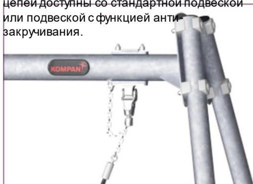
KOMPAN heavy duty designed swing hangers of stainless steel with anti-twist function. The moving parts of the swing hanger is lifetime sealed and lubricated. The hanger system is equipped with a safety chain to prevent the swing hanger to fall down if damaged.
