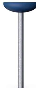
The tube of the Grasshopper is made of a  $\varnothing 48,3 \times 2,9$ mm, hot dip galvanized steel tube. The top seat is connected with a M12 bolt and covered by a PE top cap.
